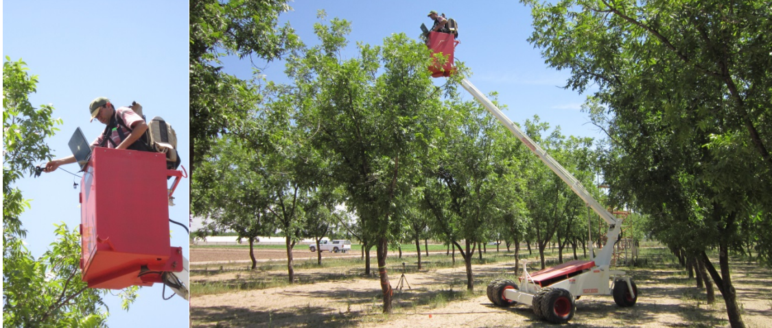
Figure 2. Canopy surface reflectance measurements using hand-held spectroradiometer (ASD Fieldspec Pro Full Range Spectroradiometer) at the leyendecker orchard.
